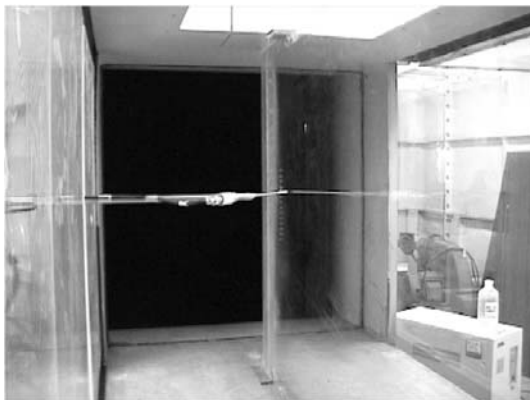
Fig. 3 Flat plate model and hot wire installed in the test section
